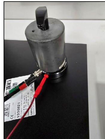
Picture 3: Measuring arrangement according ANSI/ESD STM11.11 and IEC 61340-2-3; Measurement with a concentric ring electrode R_s
